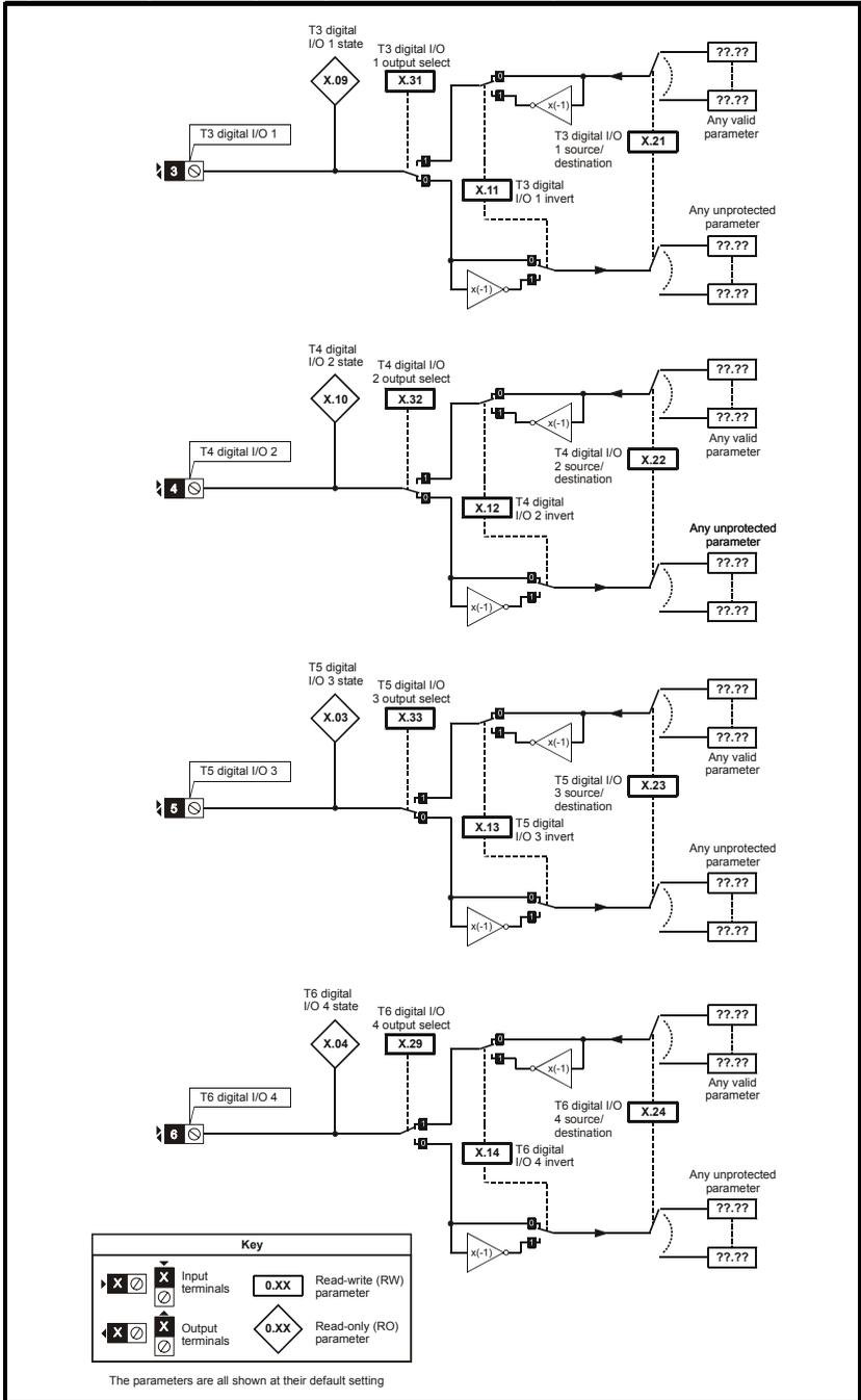
Figure 5-2 Digital I/O logic diagram (Commander SK only)
