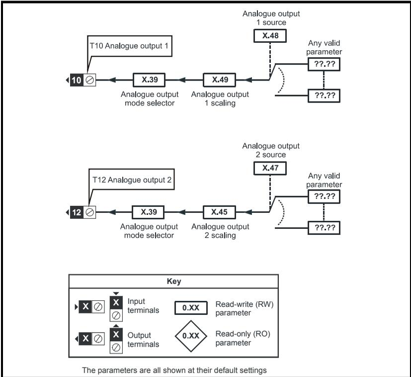
**Figure 5-8 Analogue output logic diagram (Commander SK only)**
