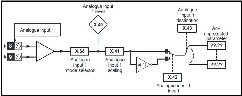
**Figure 5-6 Analogue input logic diagram (voltage mode)**
