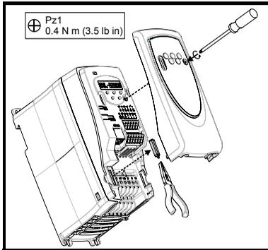
**Figure 4-4 Fitting and removing a Solutions Module into the Commander SK**
