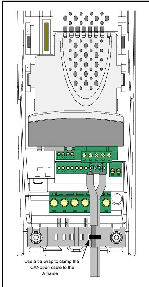
**NOTE** Care should be taken when clamping cables to avoid damage to the cable.
