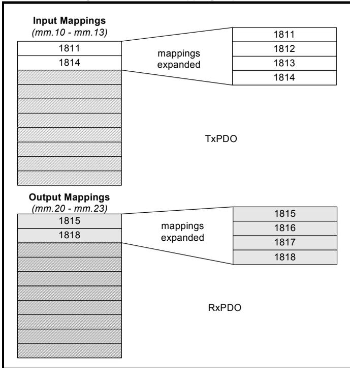
Block mapping can also be used when mapping data to the PLC registers in SM-Applications. If it is required to map to individual parameters within the same menu ensure that the target registers are listed in descending order (see section 11.6.1 *Avoiding block mapping* ).
