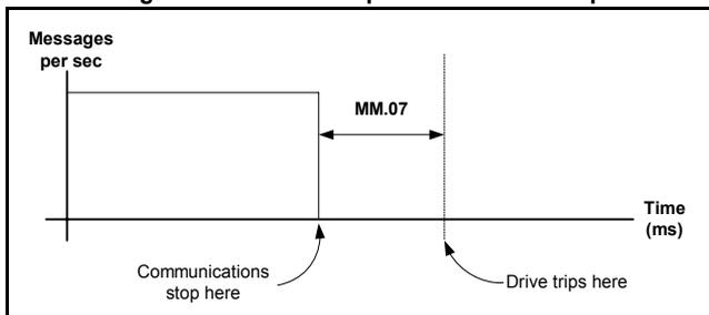
As the trip delay time is reduced, the network loss trip will occur more quickly in the event of a loss of network. However, if the network loss trip time is reduced too far, spurious network loss trips may occur due to time-out occurring before the next message has chance to arrive. The network loss trip time should be set such that a minimum of 4 messages will be received in the specified time period under normal operating conditions.
