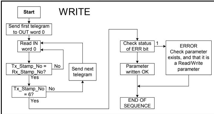
The following example telegrams show how to set the digital speed reference 1 (Pr 1.21) to 12553.9 rpm (32-bit value is 125539) in the drive.
