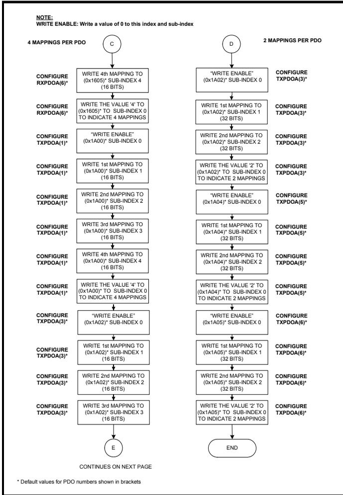
**NOTE** PDOs A,B,C & D may be configured to any valid PDO number, TxPDO and RxPDO numbers are independent. The default configuration for PDO A,B,C & D are PDO numbers 1, 3,5 & 6 respectively. the default configuration uses the same numbers for both TxPDOs and RxPDOs, although this is not a requirement.
