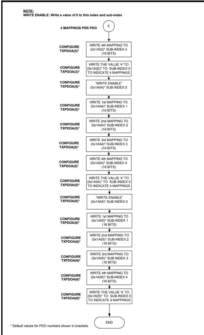
**NOTE** PDOs A,B,C & D may be configured to any valid PDO number, TxPDO and RxPDO numbers are independent. The default configuration for PDO A,B,C & D are PDO numbers 1,3,5 & 6 respectively. The default configuration uses the same numbers for both TxPDOs and RxPDOs, although this is not a requirement.
