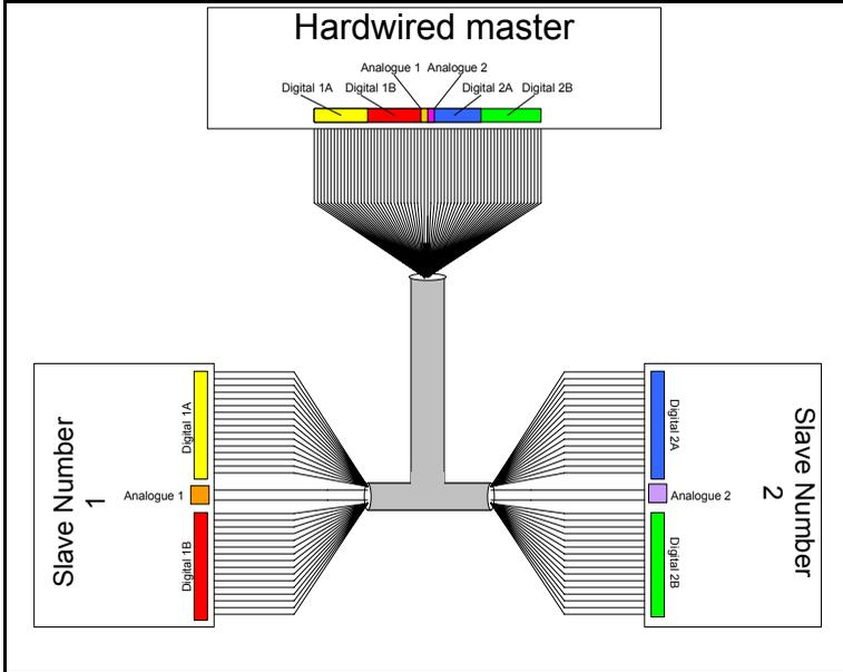
Table 2.1 details how the wiring is used to communicate data between the master and the slaves. Each signal that is communicated requires one signal wire giving a total of 66 signal wires plus a 0V return.
