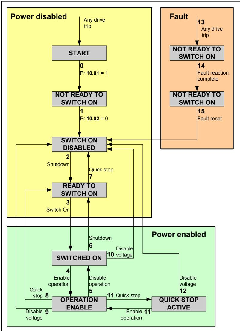
State transitions are caused by internal events in the drive or by commands received from the host via the **controlword** (refer to Figure 12-3 *controlword state diagram* on page 137).
