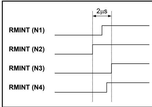
In this case, the worst case delay between RMINTs is between node 2 and node 3. The difference between any other pair of nodes is always less than 2µs.
