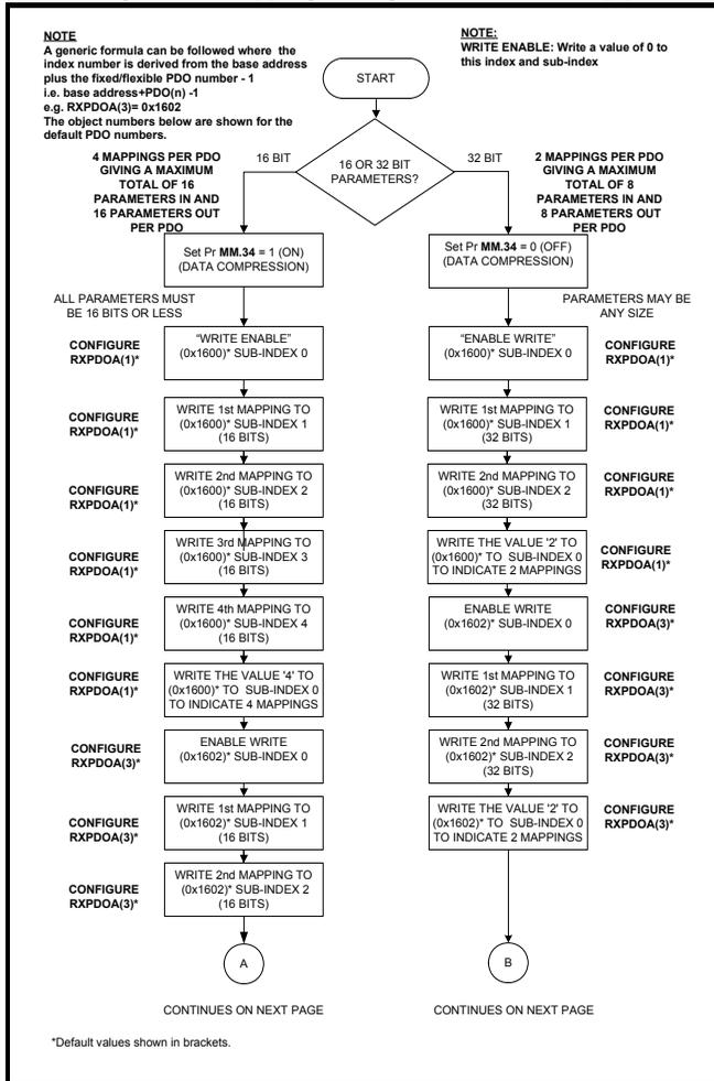
**NOTE** Setting Pr MM.34 to a 1 (data compression on) will allow a maximum of 4 mappings. If data compression is off, or the parameters are 32 bits, then only 2 mappings will be possible (i.e. each PDO has 64 bits, so the size of the parameters mapped will determine the maximum number of mappings). PDOs A,B,C & D may be configured to any valid PDO number and the TxPDO and RxPDO numbers are independent. The default configuration for PDOA, B, C & D are PDO numbers 1, 3, 5 & 6 respectively.
