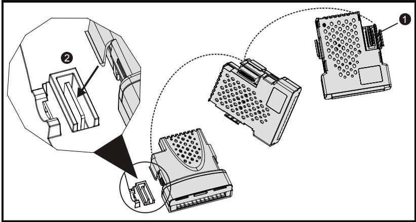
The Solutions Module connector is located on the underside of the module (1). Push this into the Solutions Module slot located on the drive until it clicks into place (2). Note that some drives require a protective tab to be removed from the Solutions Module slot. For further information, refer to the appropriate drive manual.
