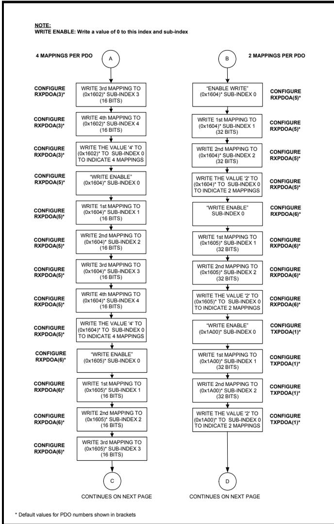
**NOTE** PDOs A,B,C & D may be configured to any valid PDO number, TxPDO and RxPDO numbers are independent. The default configuration for PDOA,B,C & D are PDO numbers 1, 3, 5 and 6 respectively, the default configuration uses the same numbers for both TxPDOs and RxPDOs, although this is not a requirement.
