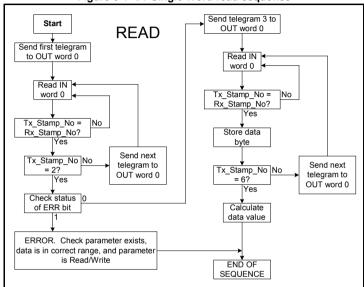
The following example telegrams show how to read the post-ramp speed reference (in rpm with 2 decimal places) from Pr **2.01** in the drive.
