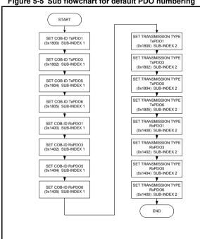
Figure 5-5 Sub flowchart for default PDO numbering
