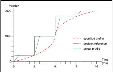
The solution is to use position reference interpolation. When a new position reference is received from the CANopen master controller, 3 intermediate step positions can be calculated and passed to the position controller on each 1ms cycle. This is shown in Figure 11-9 *Linear interpolation* where each interpolated position reference is a quarter of the position move required during the 4ms period.
