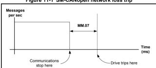
Figure 11-1 SM-CANopen network loss trip
