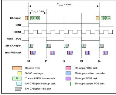
When the CANopen SYNC time is 4ms, the position reference received from the master controller is the target position that must be achieved 4ms later. If the SM-Applications position controller is running every 1ms, it will try to move to the new position in 1ms, instead of 4ms. The actual movement that will be produced is shown in section 11.14.5 *Synchronisation period* on page 89, and looks nothing like the specified profile.
