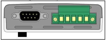
The terminals are numbered from 1-5 reading from left to right (see Figure 4-2).
